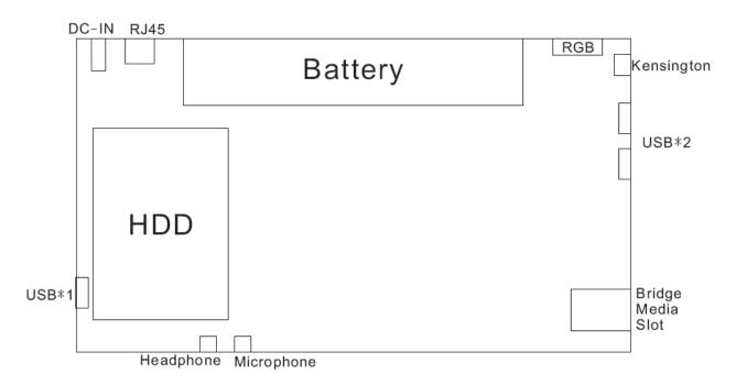
Figure 1-3 System Board Configurations
